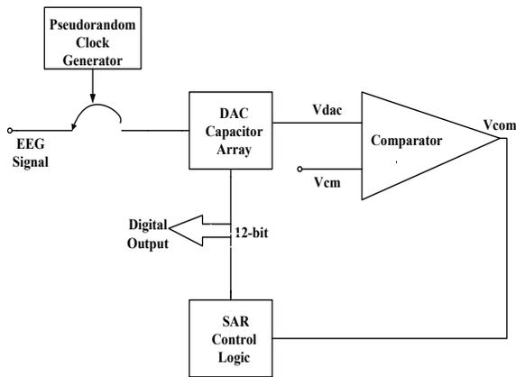
Fig. 3 Block diagram of Analog-to-Information Converter.
