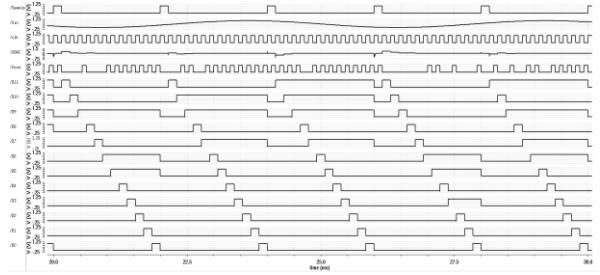
Fig. 4 Transient response of ADC.
