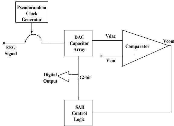
Fig. 3 Block diagram of Analog-to-Information Converter.
