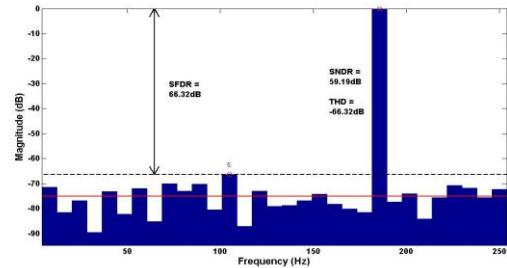
Fig. 5 AIC output spectrum.
