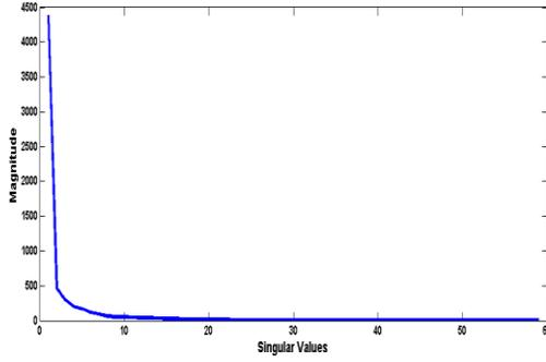
Fig. 1 Decay of singular values for multi-channel signal ensemble.
