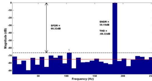
Fig. 5 AIC output spectrum.
