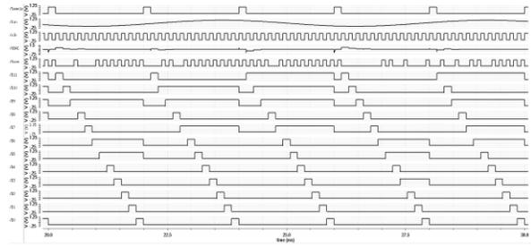
Fig. 4 Transient response of ADC.
